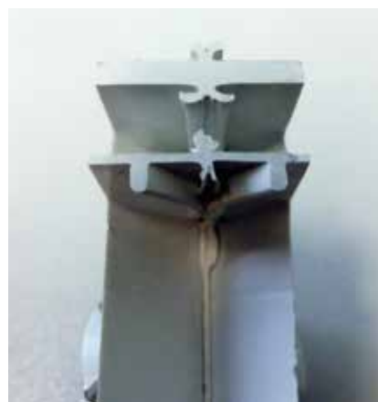
Fig. 12: Profile section showing bead limitation (l.) | Bead limitation in the welding machine (r.)
