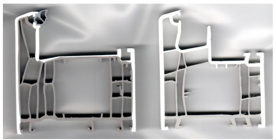
Figure 1: Profile cross section with a recyclate core (grey, about 40%). The left profile also contains recyclate in the external wall, thereby increasing the recyclate content to over 40%.
